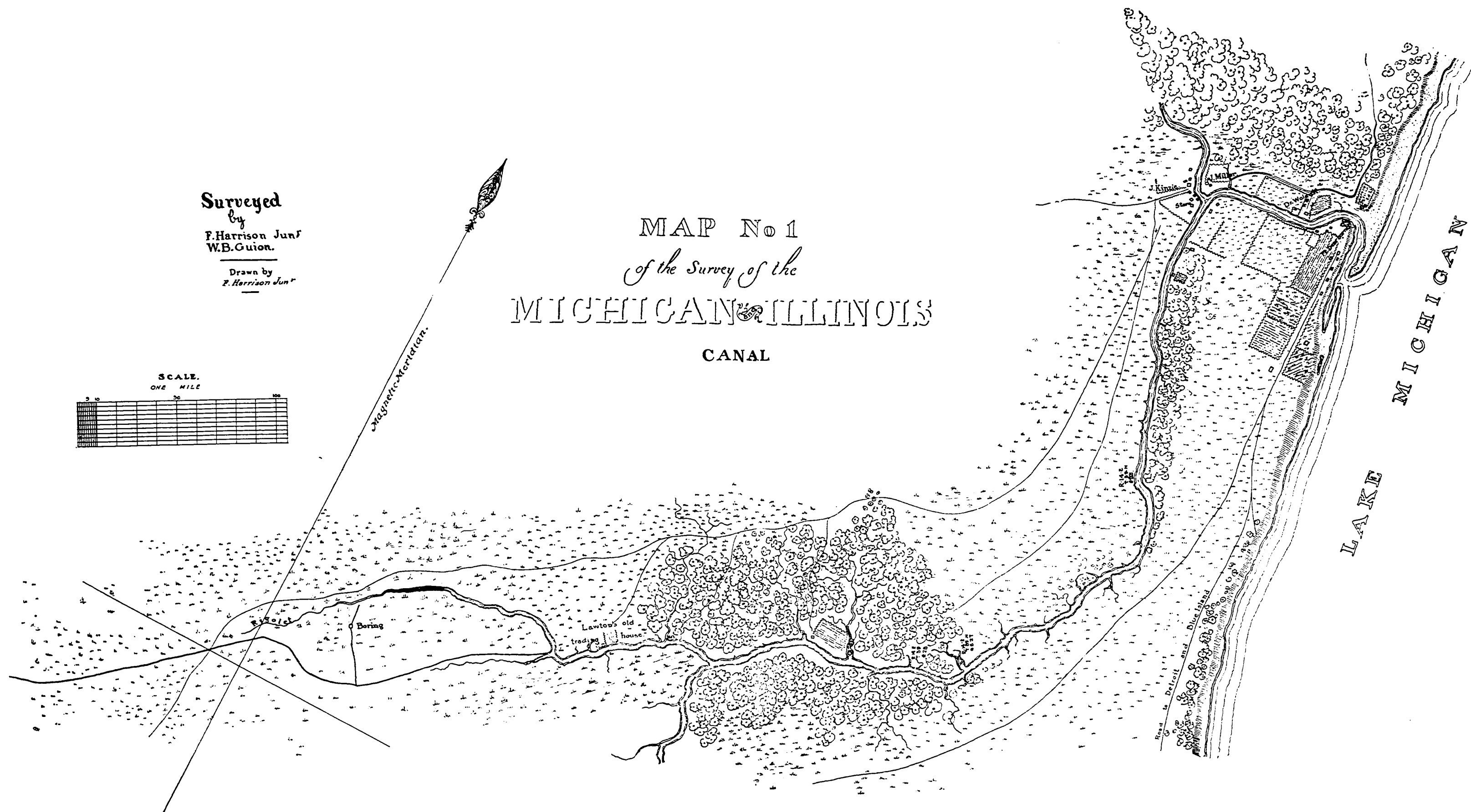
Map of a survey of the Chicago River made in 1829 by Harrison and Guion, United States engineers. The early trails leading to and from Fort Dearborn are shown together with the buildings of pioneer settlers and traders. The location of "Lawton's old trading house" shows prominently near the head of navigation indicated by a black line in the course of the river. This building probably occupied the site of Père Marquette's cabin of 1674-5. The Lawtons moved from this location to the Des Plaines River. (See page 69.)
